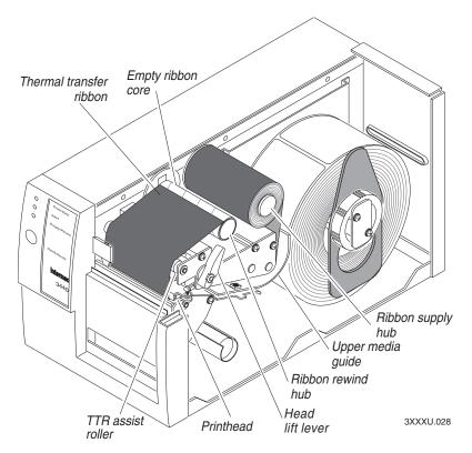
**5** Route the ribbon leader through the printer mechanism as shown in the previous illustration.
